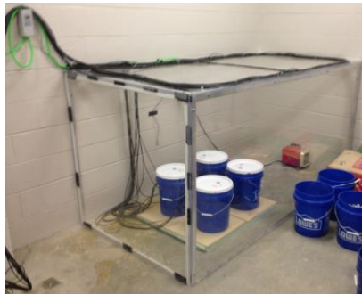
Figure 4.3 Test setup. Controlled temperature chamber (left) and specimens placed in 100% relative humidity buckets (right).
