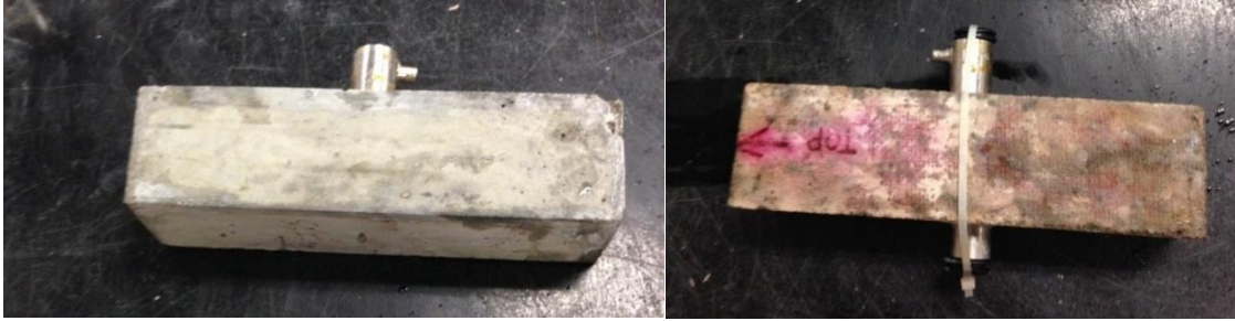
Figure 4.6 Photograph of control specimen (C1-365, left) and ASR specimen (S10-365, right) after 365 days of exposure.
